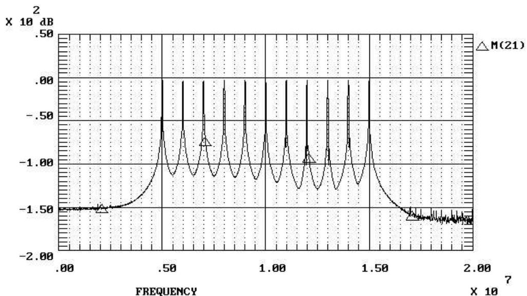
Figure 1.6: A typical frequency hopping spectrum
