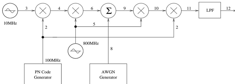
Figure 1.13: System diagram showing the addition of AWGN
