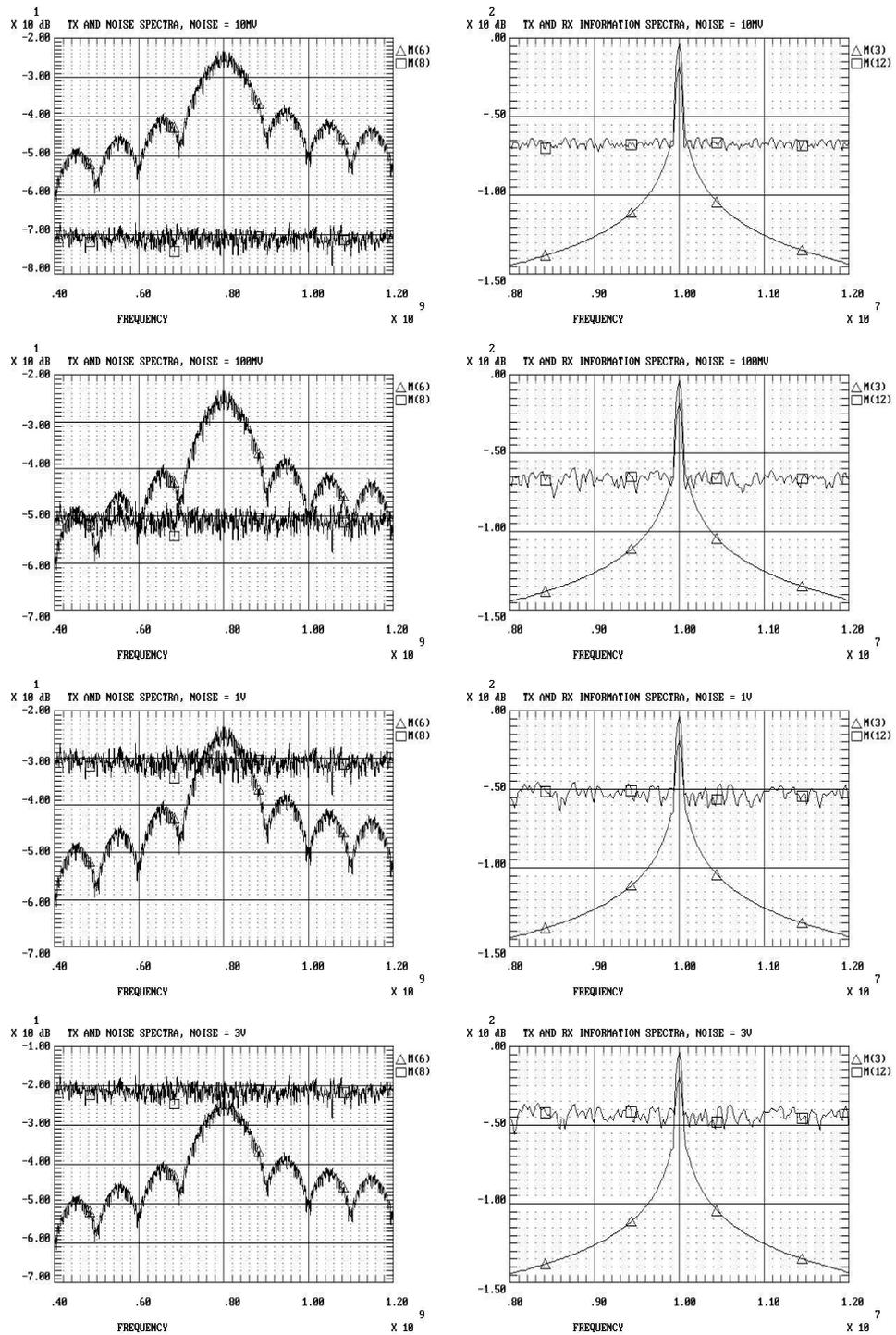
Figure 1.14: Transmitted spectrum with recovered signal under the influence of varying noise levels
