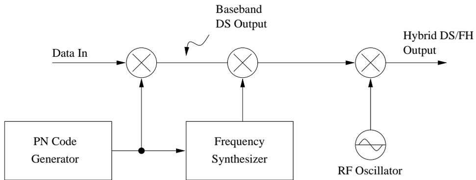
Figure 1.9: Hybrid DS/FH spread spectrum transmitter
