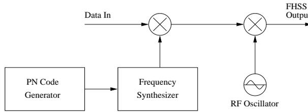
Figure 1.7: Frequency hopping spread spectrum transmitter
