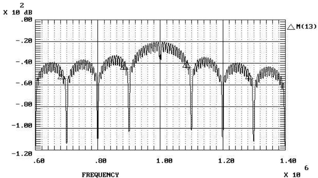
Figure 1.2: A typical direct sequence spectrum
