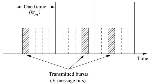
Figure 1.11: A typical time hopping waveform
