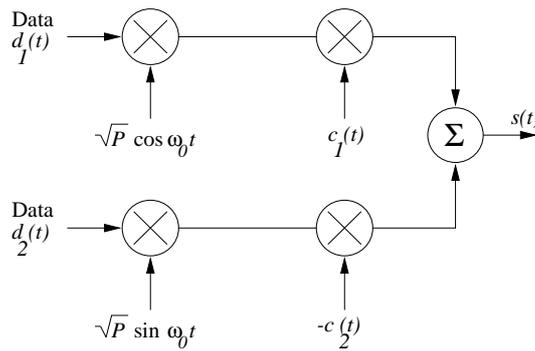
Figure 1.5: Quadrature phase modulated DS transmitter
