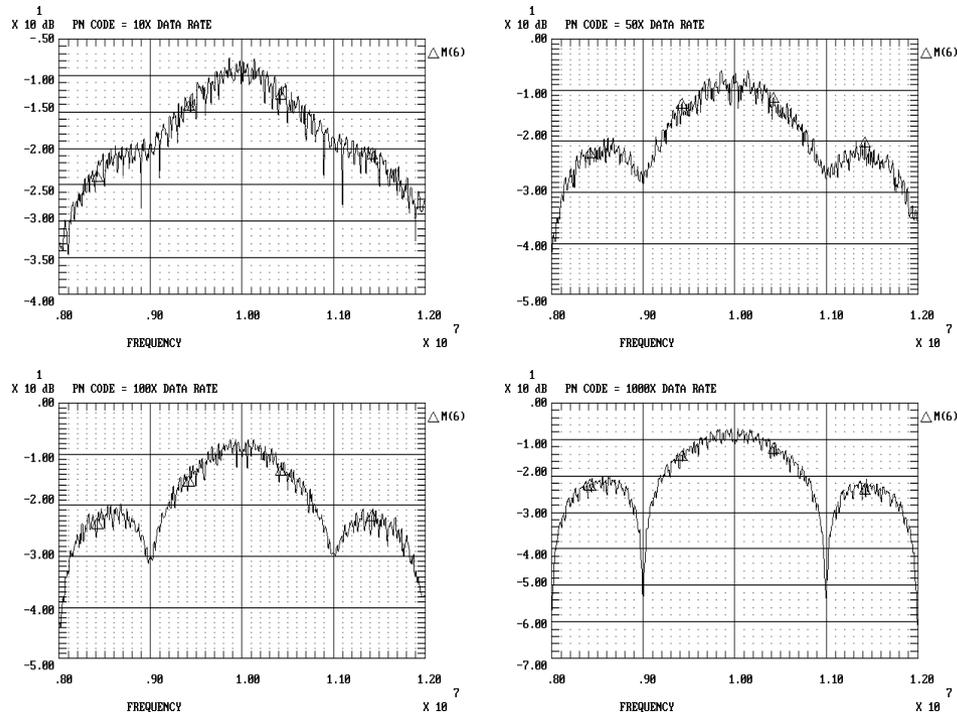
Figure 1.12: The effect of varying the processing gain
