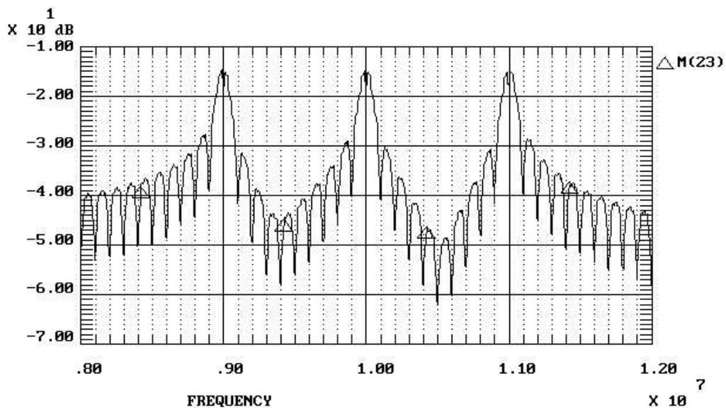
Figure 1.10: Spectrum of a hybrid DS/FH system
