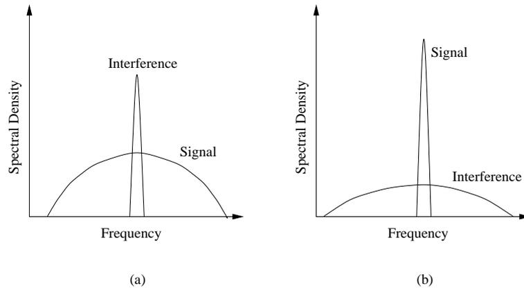
Figure 1.4: Effect of de-spreading: (a) Spectra before PN multiplication and (b) after multiplication
