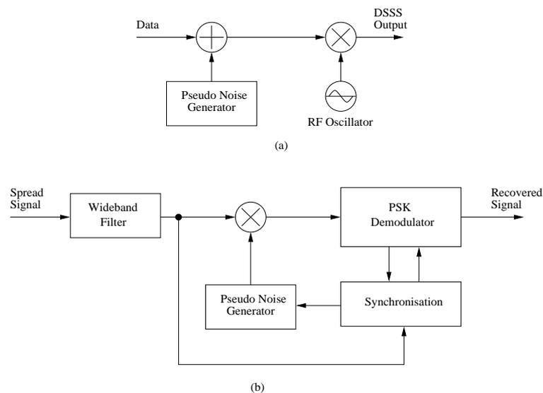
Figure 1.1: Binary phase modulated direct sequence system, (a) Transmitter and (b) Receiver
