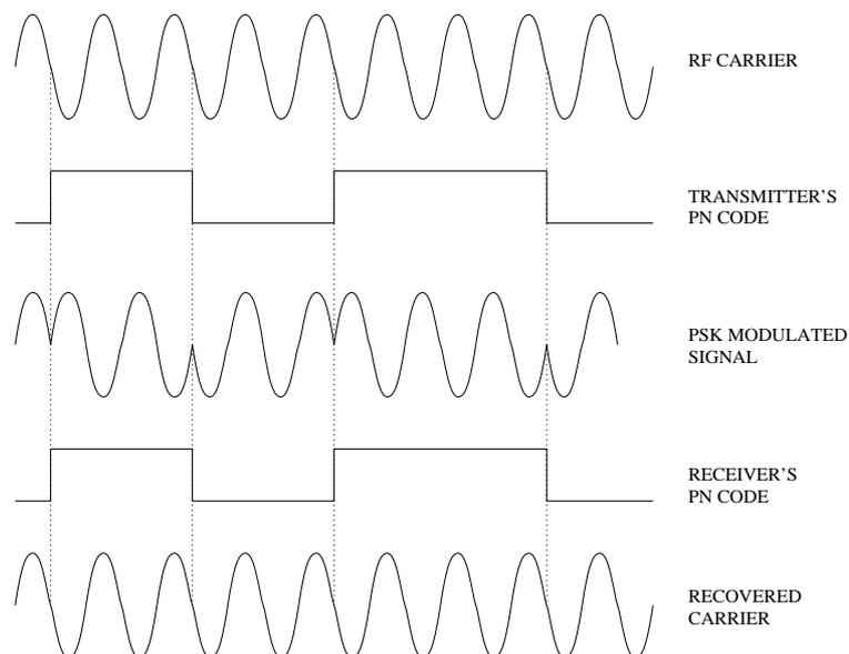
Figure 1.3: Carrier recovery using an in-line correlator
